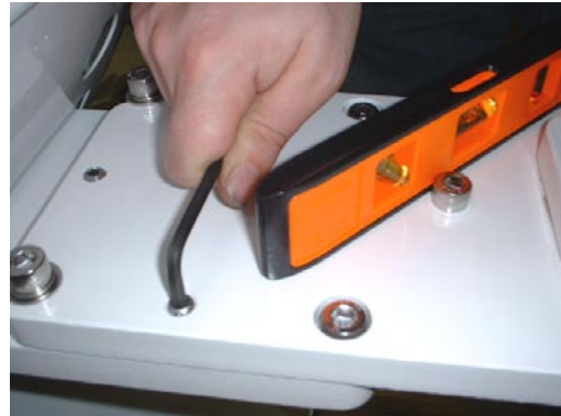
Adjusting leveling Set Screws for rough leveling of Swing Arm Assembly without Umbilical Bracket attached
