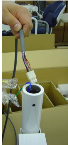
Feed Touch Pad Wire Harness down through Swing Arm.
