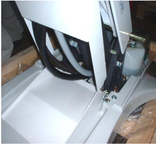
Umbilical and hoses are routed between the relay box and pump to the location of the J-Box.
