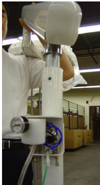
Mount Balance Arm onto Swing Arm.
