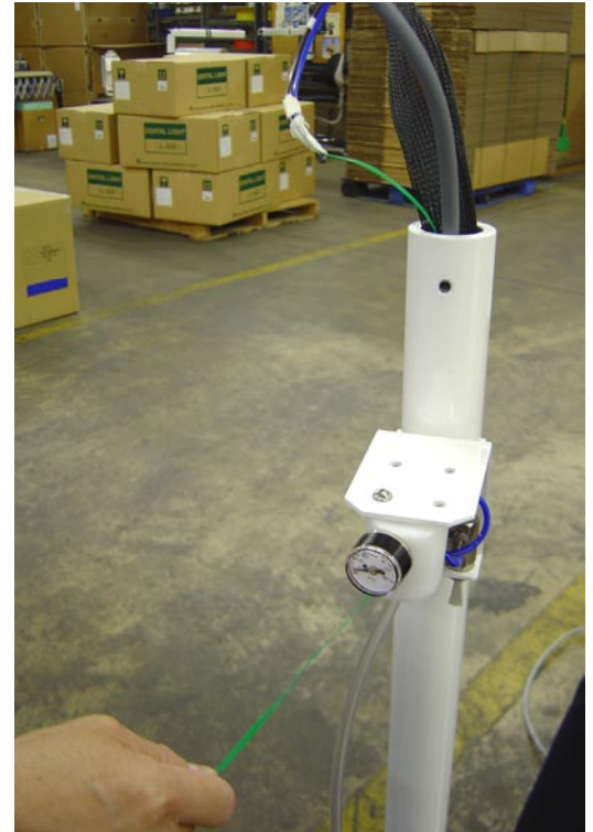
Mount Doctor Table/ Balance Arm Assembly to Swing Arm. Feed umbilical and touchpad wire harness downward and gradually pull green flexible ribbon attached to ends of 1/8" brown & 1/8" blue tubing through hole in Water Bottle Mounting Bracket.
