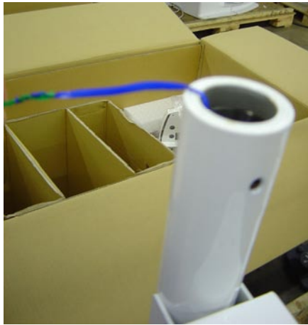
Pull flexible ribbon wire with blue & brown tubing from unit umbilical down & out through the routing hole of the Water Bottle Mounting Bracket.
