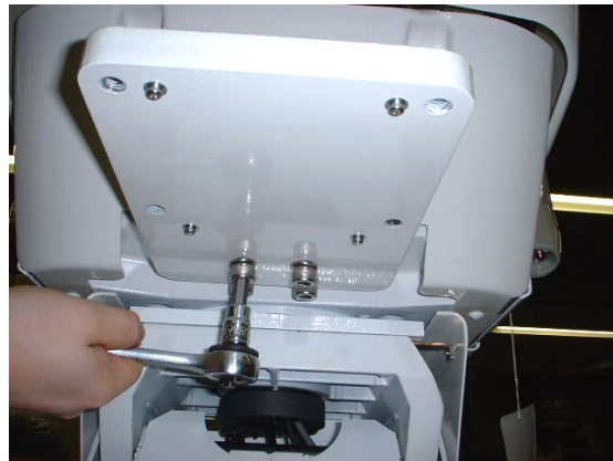
Swing Mount Bracket attaches below the AcuTrac seat casting
