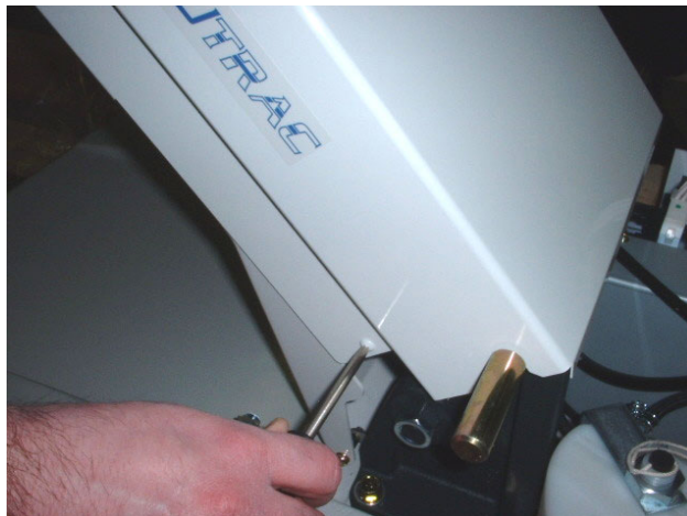
Removing the Phillips screws to release the sub-link cover and the safety shut-off plate.
