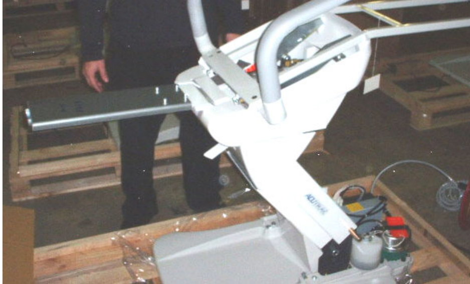
AcuTrac chair is raised to the upper limit of travel. The backrest is fully reclined to relieve spring tension.
