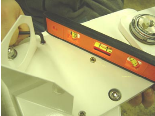
Adjusting leveling Set Screws for rough leveling of Swing Arm Assembly with Umbilical Bracket attached
