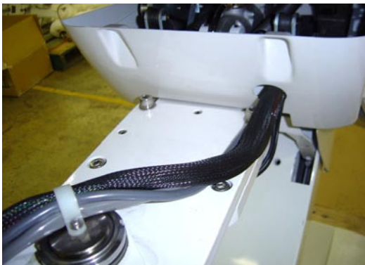
Routing umbilical through hole cut-out into the chair. Note: Umbilical shown secured to Swing Arm Pivot using C-clamp provided.
