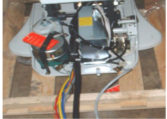
Umbilical and hoses are routed under the lift arm pivot. A cable tie may be used to secure the hoses to the side of the sub-link arm. Note: safety plate is in the down position.
