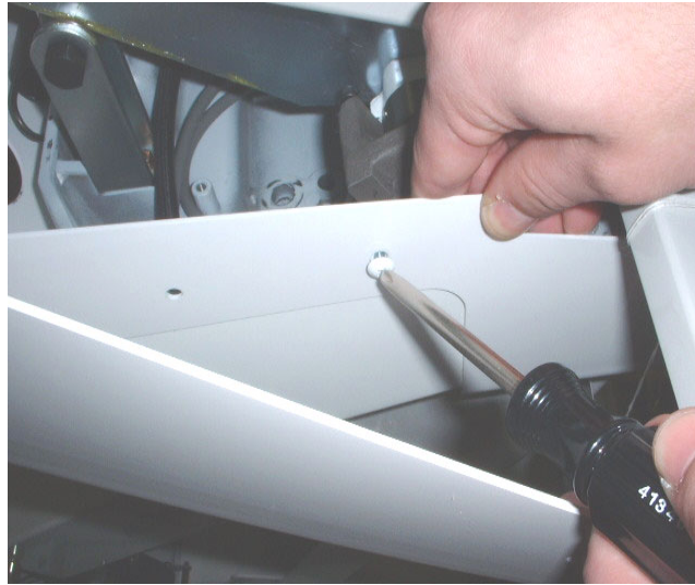
Removing the side cover plate to reveal chair adapter mounting area.
