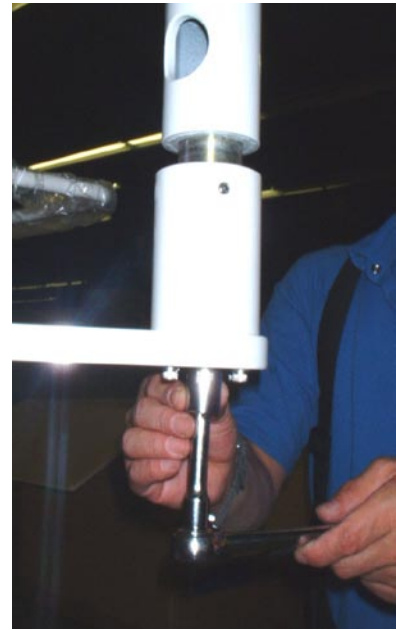
Tightening the long bolt into the unit mounting post.
