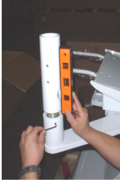
Repeat leveling at 90° to original position and tightening hub set screws.
