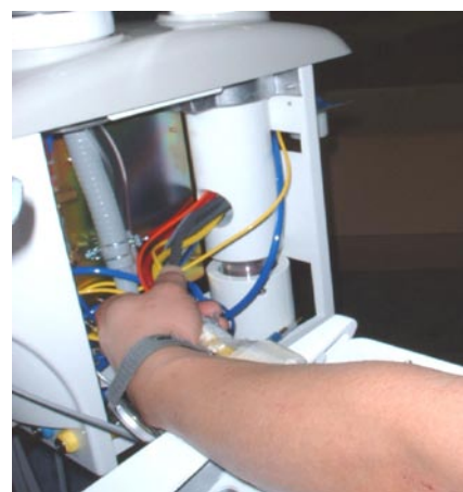
Pulling the upper umbilical tubing into the PMU.
