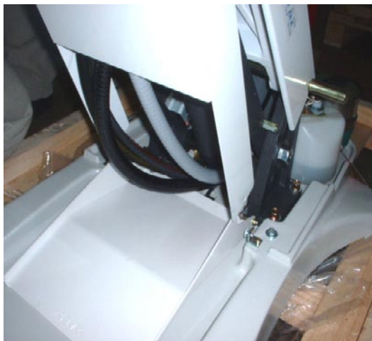
Umbilical and hoses are routed under the lift arm pivot. A cable tie may be used to secure the hoses to the side of the sub-link arm. Note: safety plate is in the down position.
