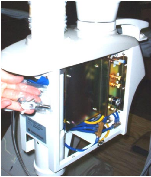
Socket cap screws are taped to the top of the water system bracket prior to shipment from the factory. (Blue tape)
