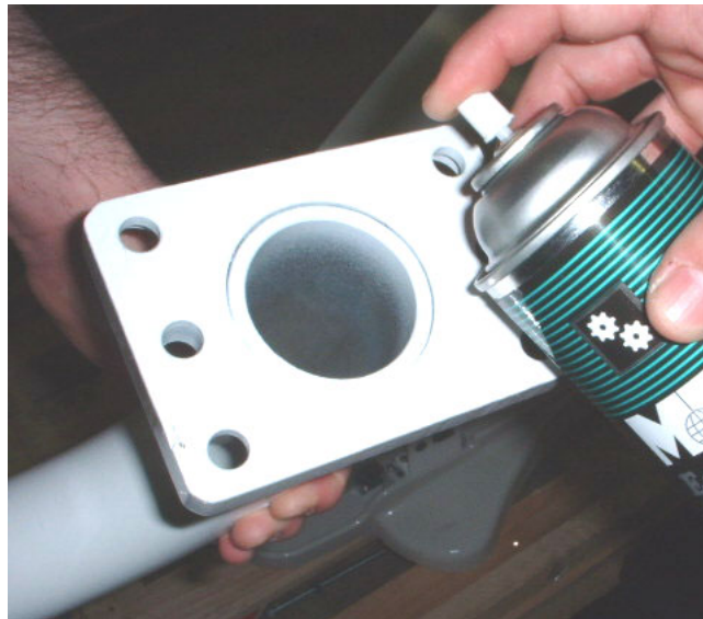
Spray silicone into chair adapter prior to umbilical insertion and mounting to the side of the chair.
