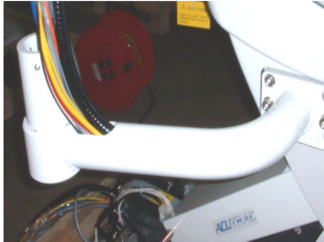
Umbilical and hoses exit the top of the chair adapter pipe.
