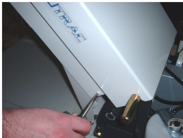
Removing the Phillips head screws to release the sub-link cover and the safety shut-off plate.
