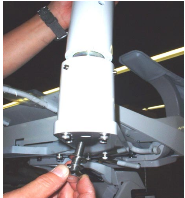
Inserting the long bolt spring and flat washer into the bottom of the chair adapter and unit mounting post.
