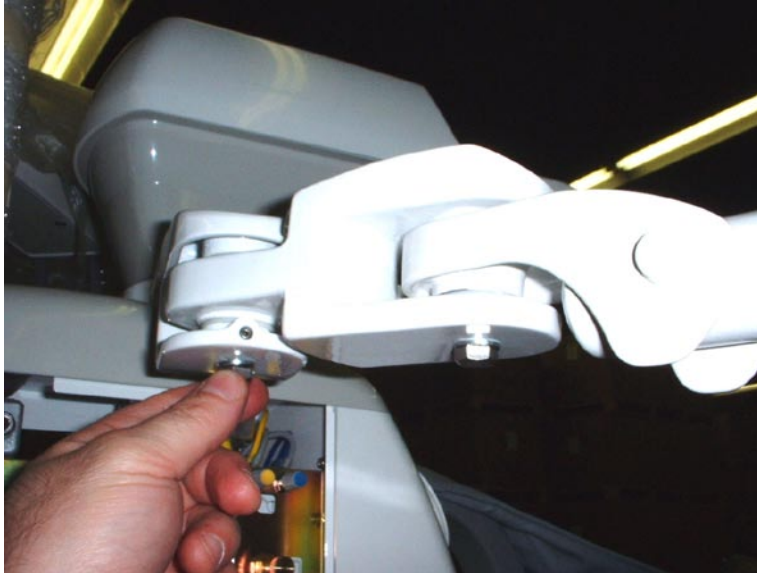
Tightening the bolt to secure the telescoping arm to the assistant rotation adapter.
