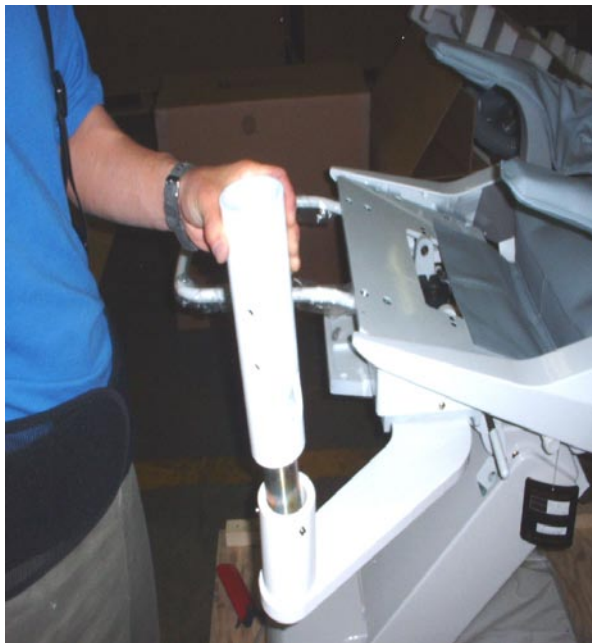
Unit mounting post insertion into the hub of the chair adapter.
