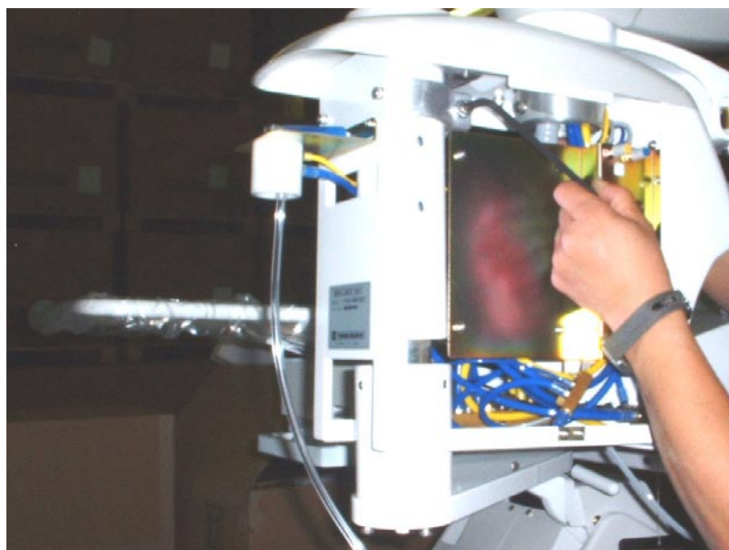
Tightening the PMU mounting clamp to the unit mounting post.
