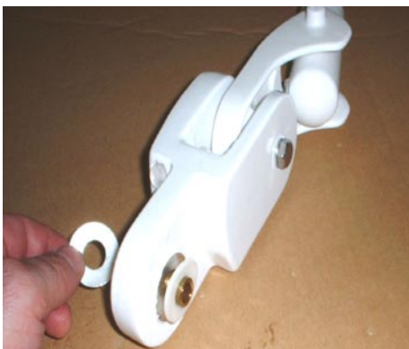
The brass bushing is inserted through the telescoping arm joint. A plastic washer is placed over each end of the bushing.
